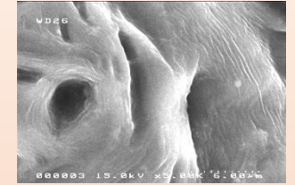
SEM micrographs of PE-based electrolyte film with Al 2 O 3 < 50 nm
